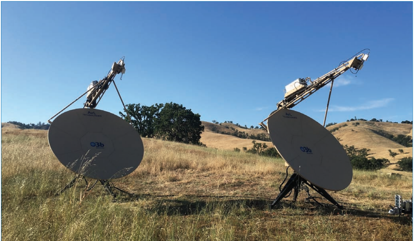
O3b 2.4m antennas operating in California. Photo courtesy Hung Tran, O3b Networks
